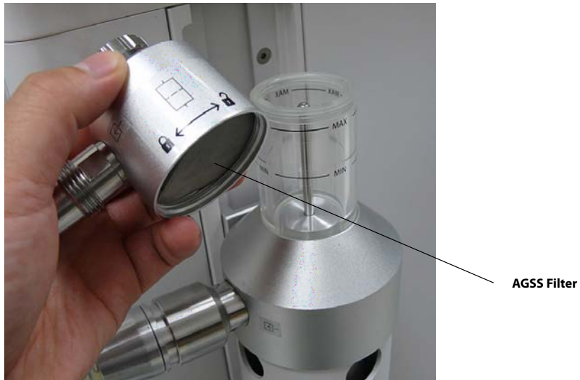
FIGURE 7-26 Removal of AGSS Top / AGSS Filter Inspection
