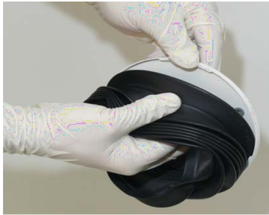
FIGURE 7-7 Detaching the Bellows Top Plate
